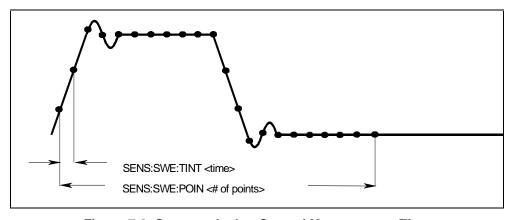
Figure 7-2. Commands that Control Measurement Time
